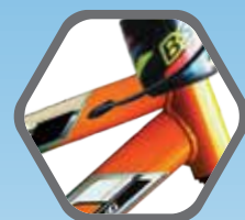
IBR - Internal Brake Routing
